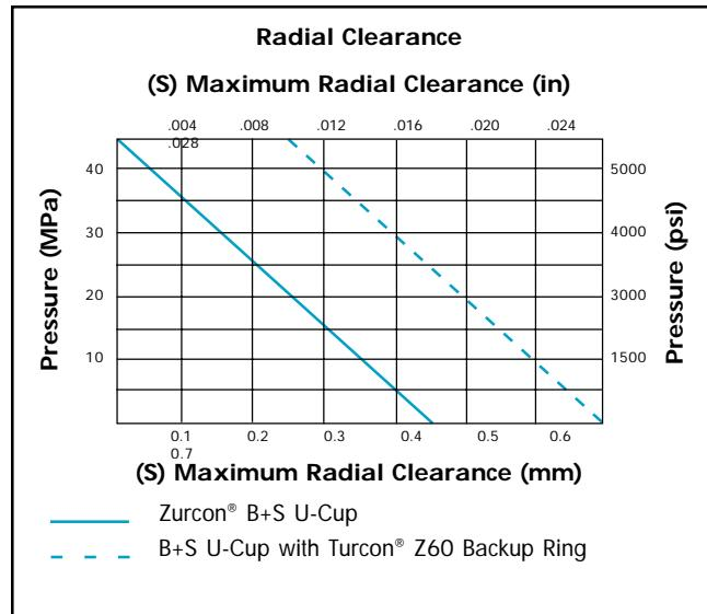
Figure 4 Relationship between radial clearance and operating pressure
