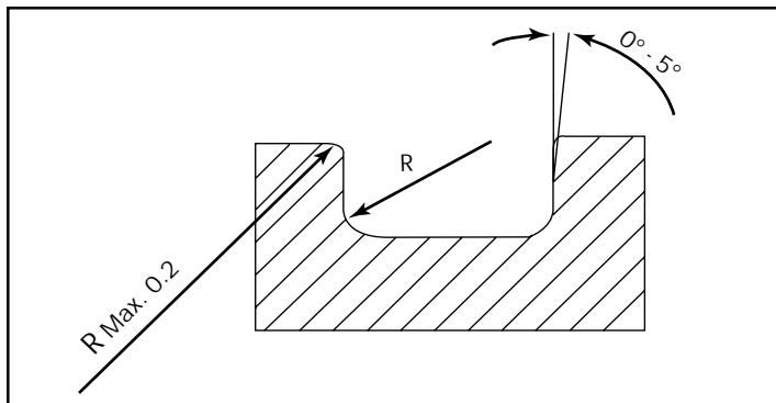
Figure 31 Groove specifications
