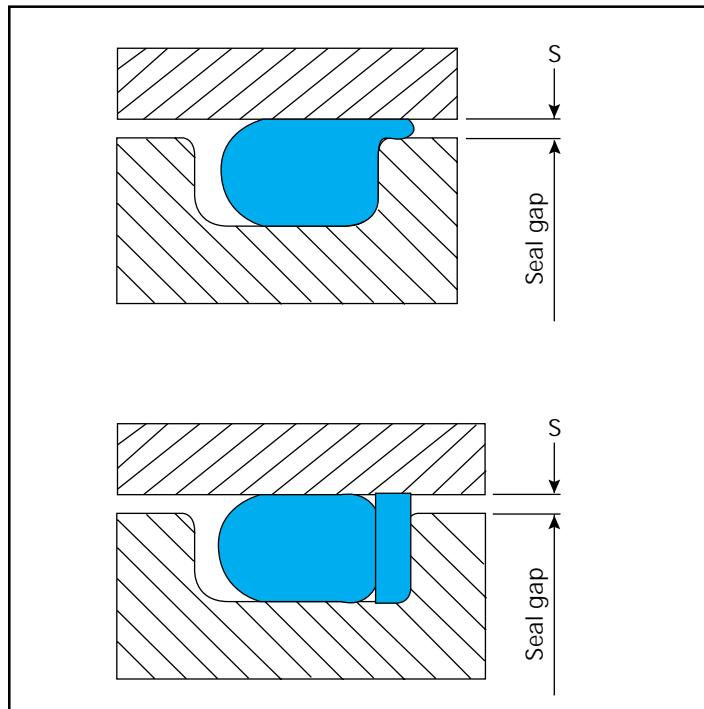
Figure 41 O-Ring installation with and without Back-up Ring
