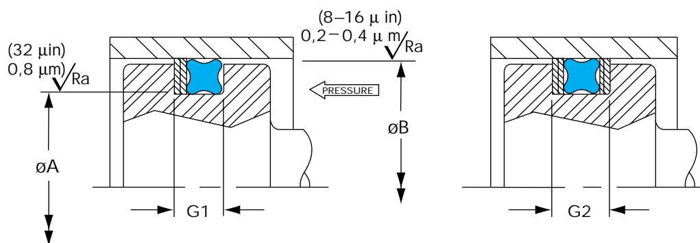
**Table 46 QUAD-RING® Seal Ordering Information for Reciprocating Piston Sealing (Metric)**
