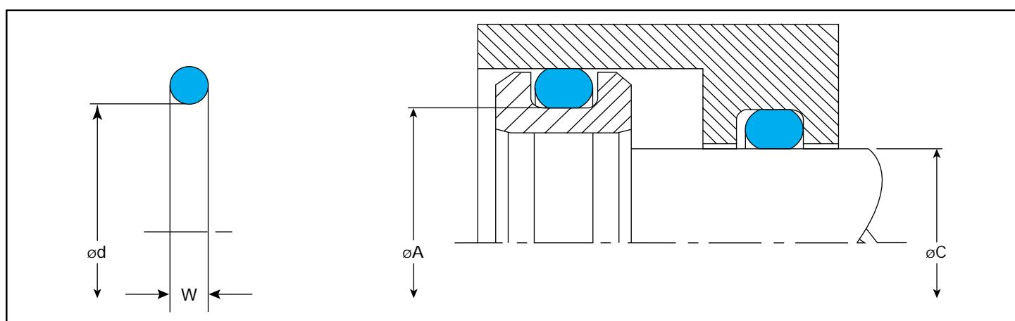
Figure 29 Radial installation
