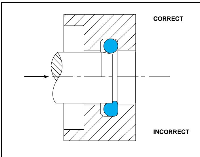
Figure 36 Rod installation with O-Ring
