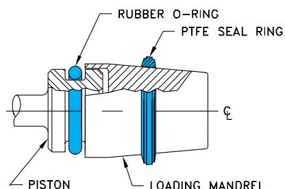
Figure 47 Piston installation
