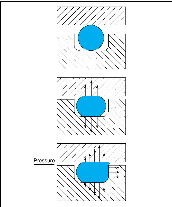
Figure 24 O-Ring sealing forces with and without system pressure
