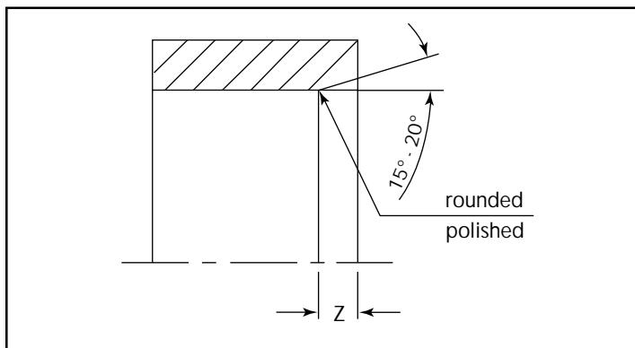
Figure 32 Lead-in chamfers for bores, tubes
