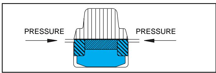
Figure 3 Turcon® CST™ Seal load distribution profile
