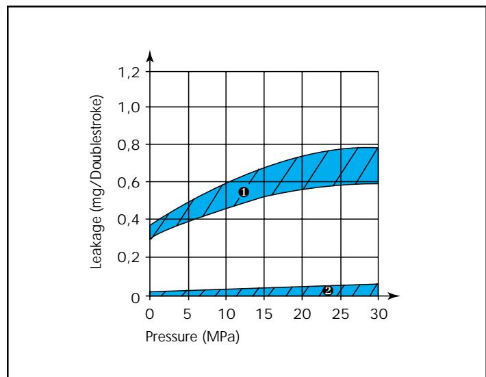
Figure 6 1) O-Ring with two Back-up rings
