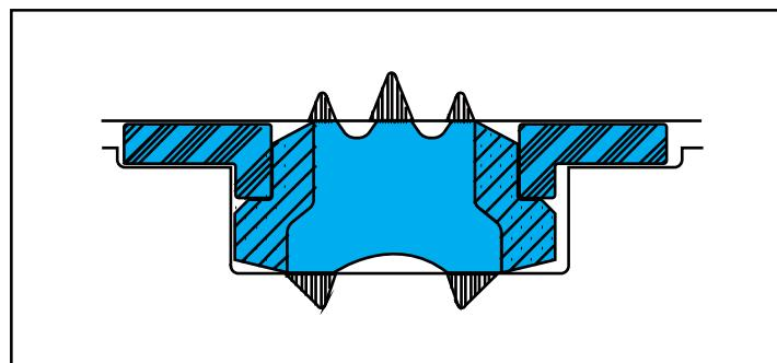
Figure 2 D-A-S Compact Seal load distribution profile
