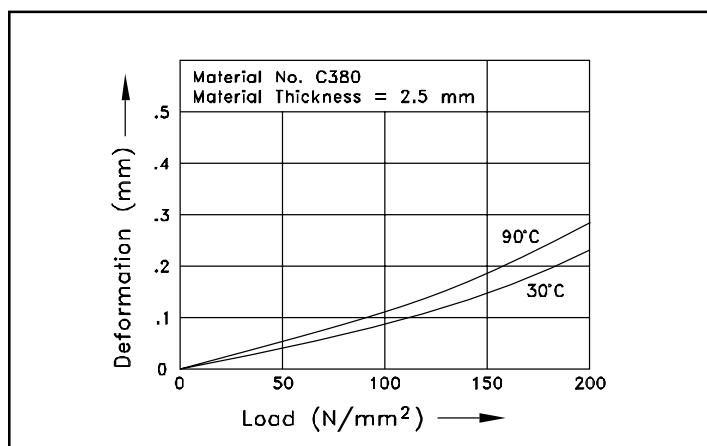
Figure 44 Deformation graph: Luytex® C380
