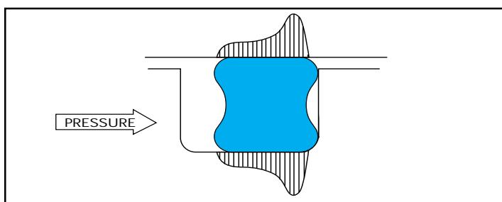
Figure 19 QUAD-RING® Seal load distribution profile
